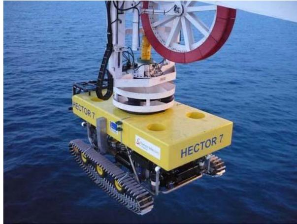
Figure 6.1: SIMEC Technology’s HECTOR-7 ROV used on Orange Marine’s Pierre de Fermat, SIMEC Technologies 2014
