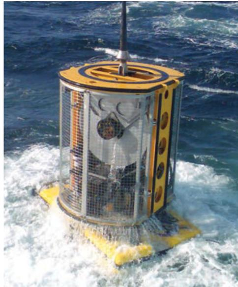
Figure 6.4: A top-hat tether management system attached to the top of an ROV, SMD 2016
