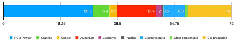
Figure 4.8: Equivalent carbon breakdown for a NCM11 battery pack (kg CO<sub>2</sub>e/kWh), Melin 2019; Dai et al. 2019
